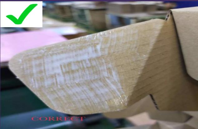
1. Apply just a thin layer of glue in the gluing portion of the item.
