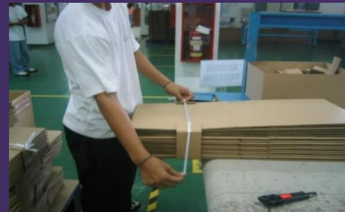
2. CB Flute, Two joint - items for inspection shall be stacked with eperan spacer between each box by the gluing operator. QA inspector/ line leader shall be informed immediately by Production before running or processing the item for the eperan spacer requisition of QA to Production.
