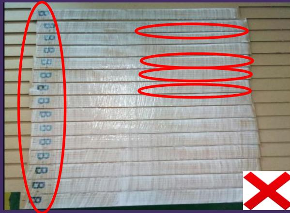
Based on the illustration, the other part of the glue tab is not filled with glue and the other part is too much. If that's the case, it can cause weak glue, glue stain and peel off.
