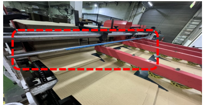
SLANTING OF ITEM HAPPENED IN THIS PORTION OF SD1800 THAT CAUSED TEAR OFF
