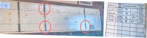
DIE-BLADE ALREADY HAVE STEEL BACKING TAPE ATTACHED WITH A SETUP PRESSURE OF 95 AND TOTAL OF 33,096 SHOTS
