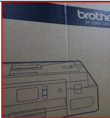
**ACTUAL:** Heavy scoring end to end on class A surface**REQUIREMENT:** Acceptable 1 pc light scoring regardless of size (no whitening; no damaged text & images)
