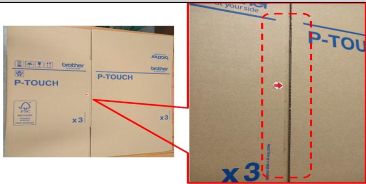
**ACTUAL:** With oil stain up to 3mm x 275mm**REQUIREMENT:** Acceptable small spot is 2mm x 3mm only
